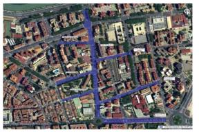
Work has been carried out on an area of 24,000 m2, comprising a total of seven streets: six paved with the innovative cool asphalt (Monte Carmelo St, Sauce St, Carmen Conde St, Valle Inclán St, Pío Baroja Avenue and Pintor Almela Costa St) and one (Lope de Rueda St) paved with the traditional one in order to be able to compare measured data.
